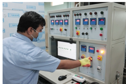
Electrical Safety Test Machine
